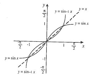
The inverse Sine Function is denoted by  $\sin^{-1} x$  and read as sine inverse x or arc sine x or sine to the minus 1 of x.
