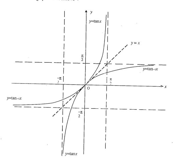
The inverse Tangent function is denoted by  $tan^{-1}x$  and is read as tan inverse x or arc tan x. In this case we restrict the angle to the open interval  $\left(-\frac{\pi}{2}, \frac{\pi}{2}\right)$ .
