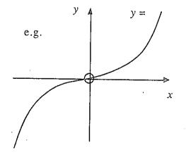
An alternative method of defining an **odd** function is to show that f(-x) = -f(x). for all values of x.
