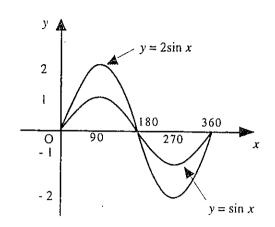
The graph of f(x) is stretched vertically if k > 1 and compressed vertically if 0 < k < 1.
